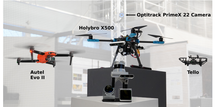
Fig. 1: Illustration of the hardware used in the experiments. At the bottom, the tracking sensors including Ouster OS1-64, Livox Mid-360, Livox Avia and Intel RealSense D435.
